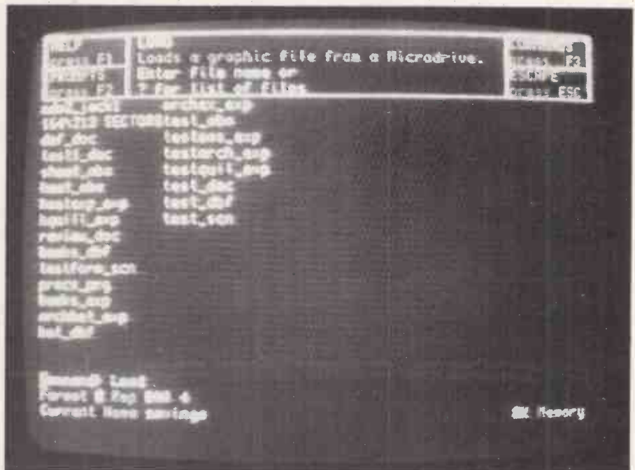
The QDOS command lists the files available on the Microdrive cartridge. The amount of free storage space left on tape is displayed in proportion to that used.
